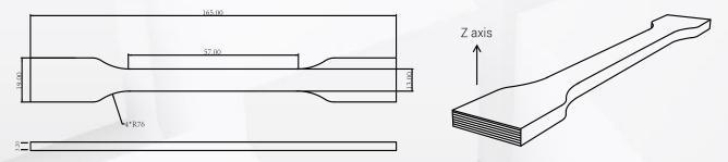
Testing prints setting: 0.1mm/layer, 100% infill, 0.4mm line width, nozzle 205°C, print surface 55°C, shells 1.2mm, speed 60mm/s.
