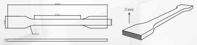
Testing prints setting: 0.1mm/layer, 100% infill, 0.4mm line width, nozzle 210°C, print surface 60°C, shells 1.2mm, speed 60mm/s.
